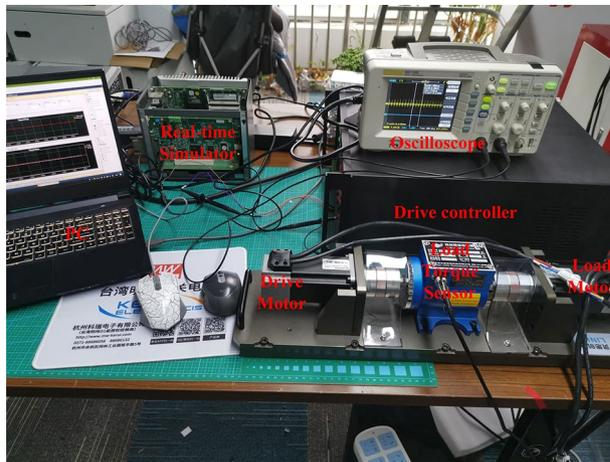
Figure 10. Experimental platform of the single-motor system.
