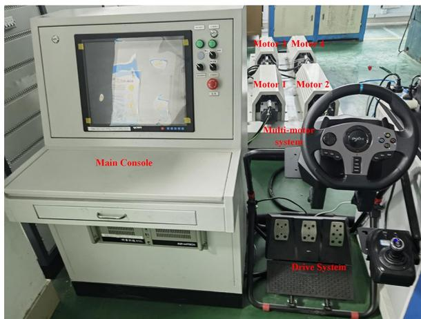
Figure 11. Experimental platform of the multi-motor system.
